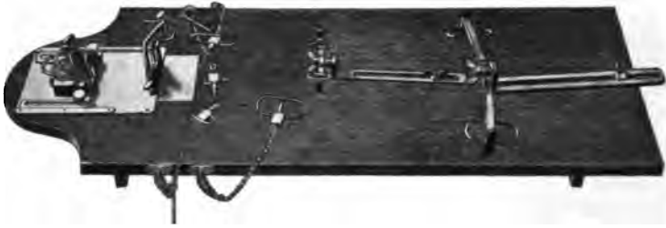
Fig. 75.—Latapie's animal holder for rabbits, guinea-pigs, and other small animals. This form of holder is in general use at the Institute Pasteur in Paris.
